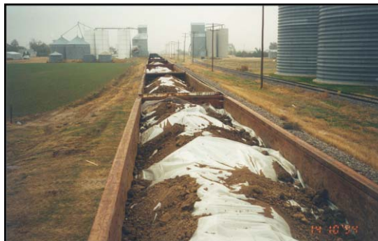
Rail cars covered in plastic and weighted down with clean soil.
