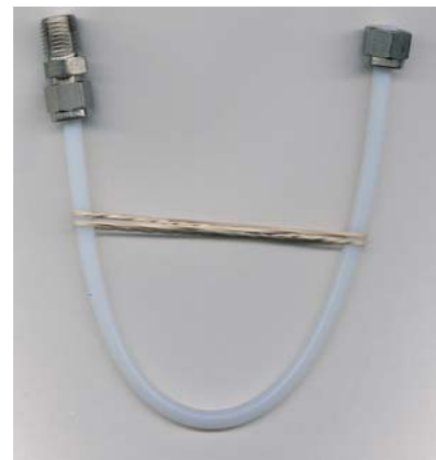
Figure 4. Tubing for collecting subslab sample
